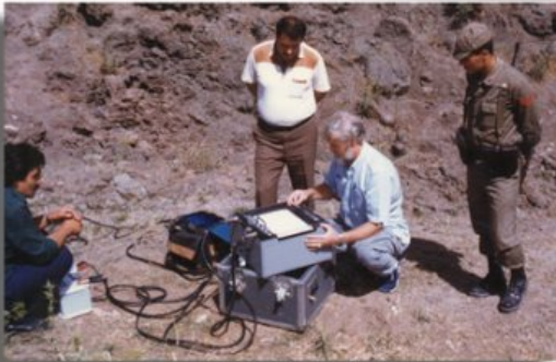
Figure 49 Radar Scans Performed with Surface Interface Radar SIR3
